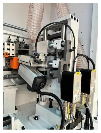
Servo precision reset to suit tape thickness from the touchscreen or program - and 4 knife TCT combi cutters - the perfect trimming setup.
