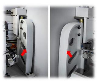
Overhead feed rollers are mounted in a heavily ribbed aluminium top beam Oversize Beam supports ensure alignment without flexing under load. A clever tensioning system guarantees parallel alignment.
