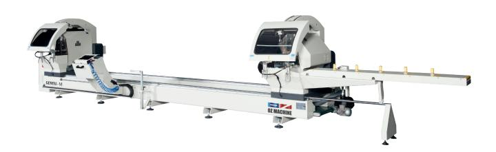
3 axis servo controlled double head cutting Machine with 550 mm saw blades **GEMINI – VI** is ideal for cutting aluminum and PVC profiles in various angles and thickness.
