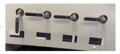
Extra sturdy guide rails with safety sensors prevent injury or damage should a stop not retract.
