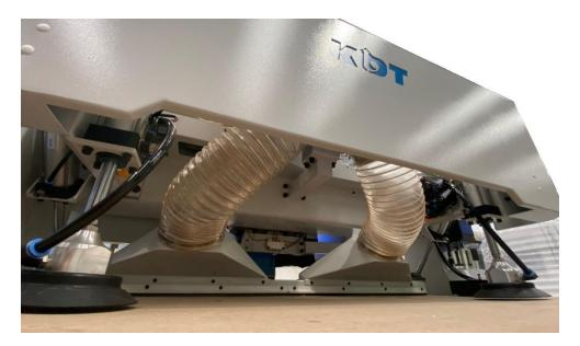
A smart unloading pusher with built in extraction pushes the completed nest to a sorting table. You can immediately load a new panel and commence your next nest effectively doubling your output.
