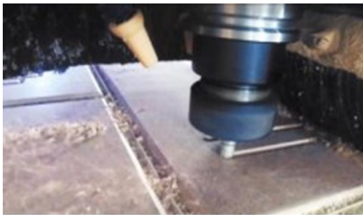
Additional blowing of the processing zone ensures effective removal of chips from the cutting zone, which significantly affects the quality of processing and tool life.
