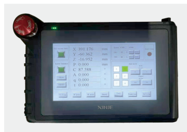
Mobile touch screen controller for easy positioning and operation with cord.
