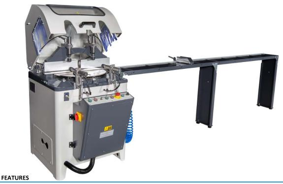
Used for cutting processes of aluminum, plastic and wooden profiles.
