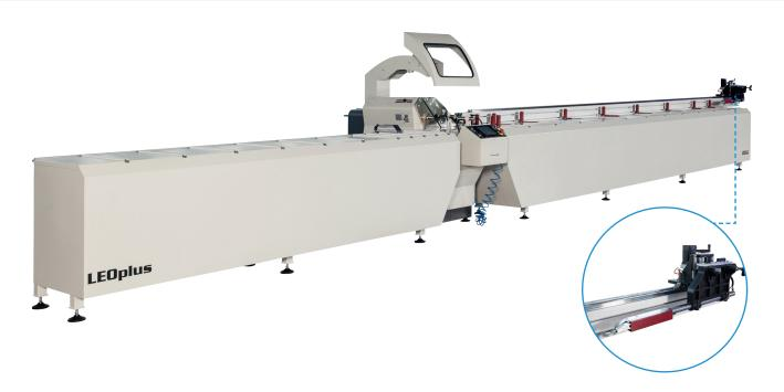
Automatic cutting machine with 550 mm saw blade **LEOplus** is ideal for cutting aluminum and PVC profiles in various angles and thickness. **LEOplus** provides rapid and precise process with servo controlled positioning of heads at any angles between -22.5° and 45° and servo controlled robotized profile loading gripper. Safety is a topmost priority for **LEOplus** together with the horizontal and vertical clamps which improve the cutting quality.
