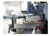
By means of the clamps that can be moved manually and is height-adjustable according to profiles, GARNET ECO III provides a flexible operating space to its users.
