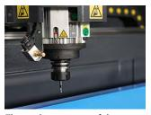
The cooling system of the automatic tool bit on the spindle motor allows you to create a clean and precise machining surface as well as it extends the service life of the tool bit.
