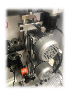
There are 2 emergency stop switches and the in-out feed of the chain feed are particularly well guarded
