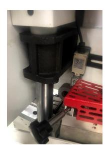
The bottom chain driven track runs on combined square and round guide rails. This is the best guide system as it ensures the track cannot move sideways or tilt under load.
