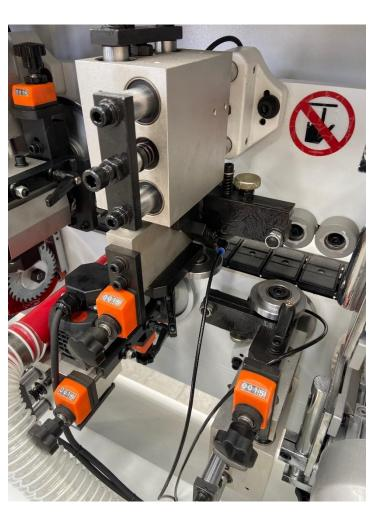
Changing from bevel to Radius is quick and easy with the combi 12 degree bevel / 2mm radius cutters.
