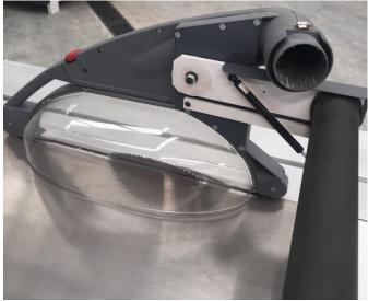
A clever slide system allows the guard to be moved clear when required.
