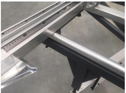
A multi chamber aluminium 100mm slide rail is kept clean with pads at both ends and supports the crosscut table with a triangular brace
