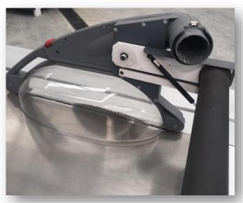
A clever slide system allows you to move the guard clear when trimming a tall cabinet or similar
