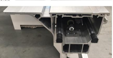
Brushes sweep the rails clean and the guiderails are set in a bevelled extrusion so dust and chips fall clear
