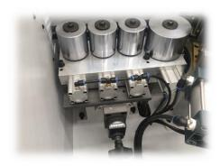
The hard chromed first driven roller does the initial application. Rollers 2 and 3 are tapered – 1 applying extra pressure at the top edge and the other at the bottom to close the glue line for a magic result. Roller 4 is the final guarantee of the perfect tight edge your customers will love. The pressure rollers are adjusted all together / digitally for different tape thickness
