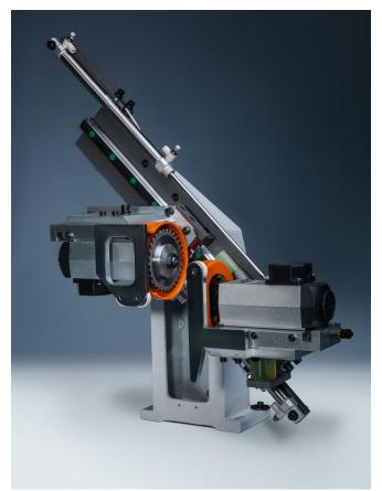
A proximity sensor works in conjunction with the line control to ensure the saws are in position before the next panel arrives — and will shut the feed down if this is not the case avoiding ruining your panel and potentially damaging the saw unit
