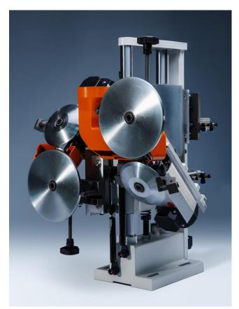
KDT use heavy steel and cast-iron construction for their Trimmer unit to guarantee the ultra-fine precision required. Large rotating '180mm copy wheels allied with 12,000 rpm HF motors ensure the cutters perfectly trace and fine trim or radius your edges prior to scraping.
