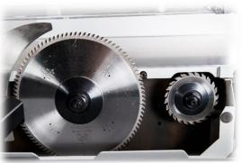
Precise height setting and locking of the Scorer blade is simple thanks to the large direct in-line adjustment on a fine thread pitch.
