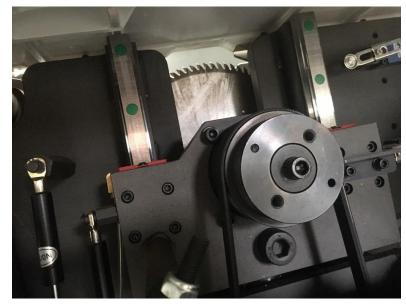
The slide ways are lubricated via a external pump maintaining smooth positioning over time.
