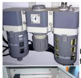
Pneumatics: Water separator and lubricator for automatic lubrication of all pneumatic machine.
