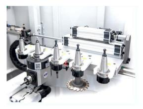
• 5 type ATC, various tool available Use for hogging, milling, lamello connector working
