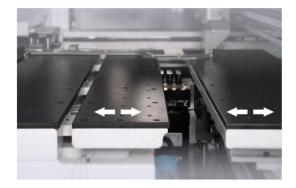
• Double translation air floatation table: can move flexibly according to the hole position to improve the drilling accuracy.
