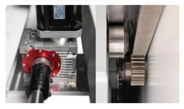
Heat treated precision rack and large diameter pinion drive for the saw carriage. Powerful 2 kw SERVO drive ensures fast, precise saw movement and positioning.
