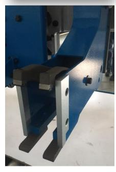
Precise pusher positioning via contact free Magnetic Strip reader
