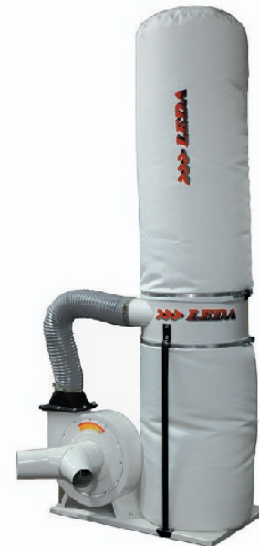
CT106 2HP Single phase 152mm inlet. 125 and 100mm adaptor. 1600 CFM
