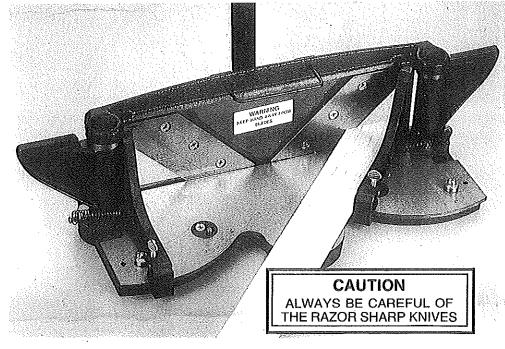
Hardwoods must be sawed at approximately 45°, then trimmed. The harder the wood, the thinner the trim cut, but the result is always a perfect miter. In off-square joinery, paper thin corrective cuts are made quickly and easily.
