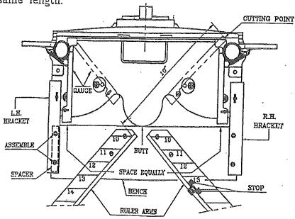
Enclosed is a small frame extension rule to be taped to the Trimmer bed for cuts down to 3".
