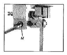
The lower blade guide is moved by loosening the socket screw(N), and turn the rear guide knob(O) to guide position is achieved.
